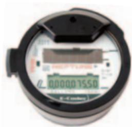
Your water meter is usually located between the sidewalk and curb under a cement cover. Remove the cover by inserting a screwdriver in the hole in the lid and then carefully lift the cover. The meter reads straight across, like the odometer on your car. Read only the black numbers (075.50).
